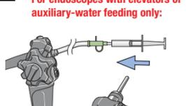
Flush detergent solution into auxiliary-water / elevator-wire channel.
