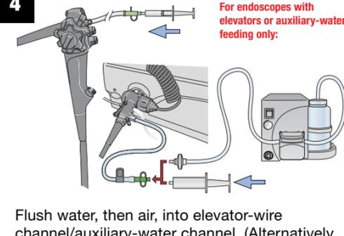
Flush water, then air, into elevator-wire channel/auxiliary-water channel. (Alternatively, the auxiliary-water channel may be flushed using the OFP pump.) The auxiliary water tube should remain attached during transport to reprocessing room.
