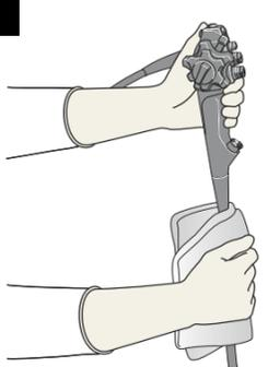
Wipe down insertion tube with a water-soaked cloth.
