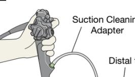
Aspirate detergent solution into suction channel.
