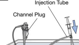
Attach injection tube and channel plug. Flush detergent solution into the air and water channels. Flush the forceps-elevator, if applicable.
