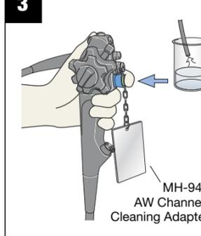
Attach AW channel-cleaning adapter. Flush water, then air, through air / water channels.
