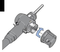
Attach water-resistant cap. This step is omitted for 190 endoscopes. Transport to the reprocessing room in a covered container. **NOTE:** Ensure that the ETO cap is removed prior to leak testing 190 generation scopes.
