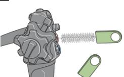
Brush the suction cylinder and instrument channel port. Repeat until all debris is removed.
