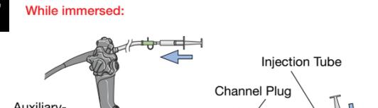
Flush clean water through all channels (including auxiliary-water / elevator-wire, if applicable). Remove from water, then flush air through all channels.
